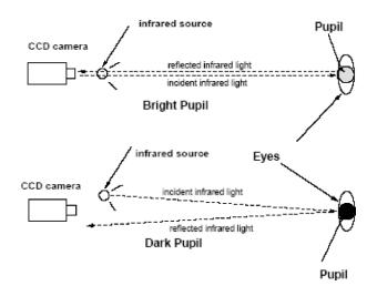
A very bright pupil can be attained if the eyes are illuminated with a NIR illuminator beaming light along the camera optical axis at a certain wavelength. At the NIR wavelength, pupils reflect nearly all IR light they admit along the path back to the camera, producing the bright pupil effect, truly important similar to the red eye effect in.photography. However, the pupils appear dark since the
